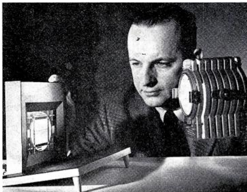
RCA's Dr. George Heilmeier demonstrates the liquid-crystal display whose image will grow stronger as the light source becomes brighter.
