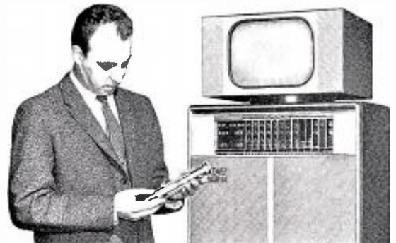
Standard transistor modules are interchangeable.
