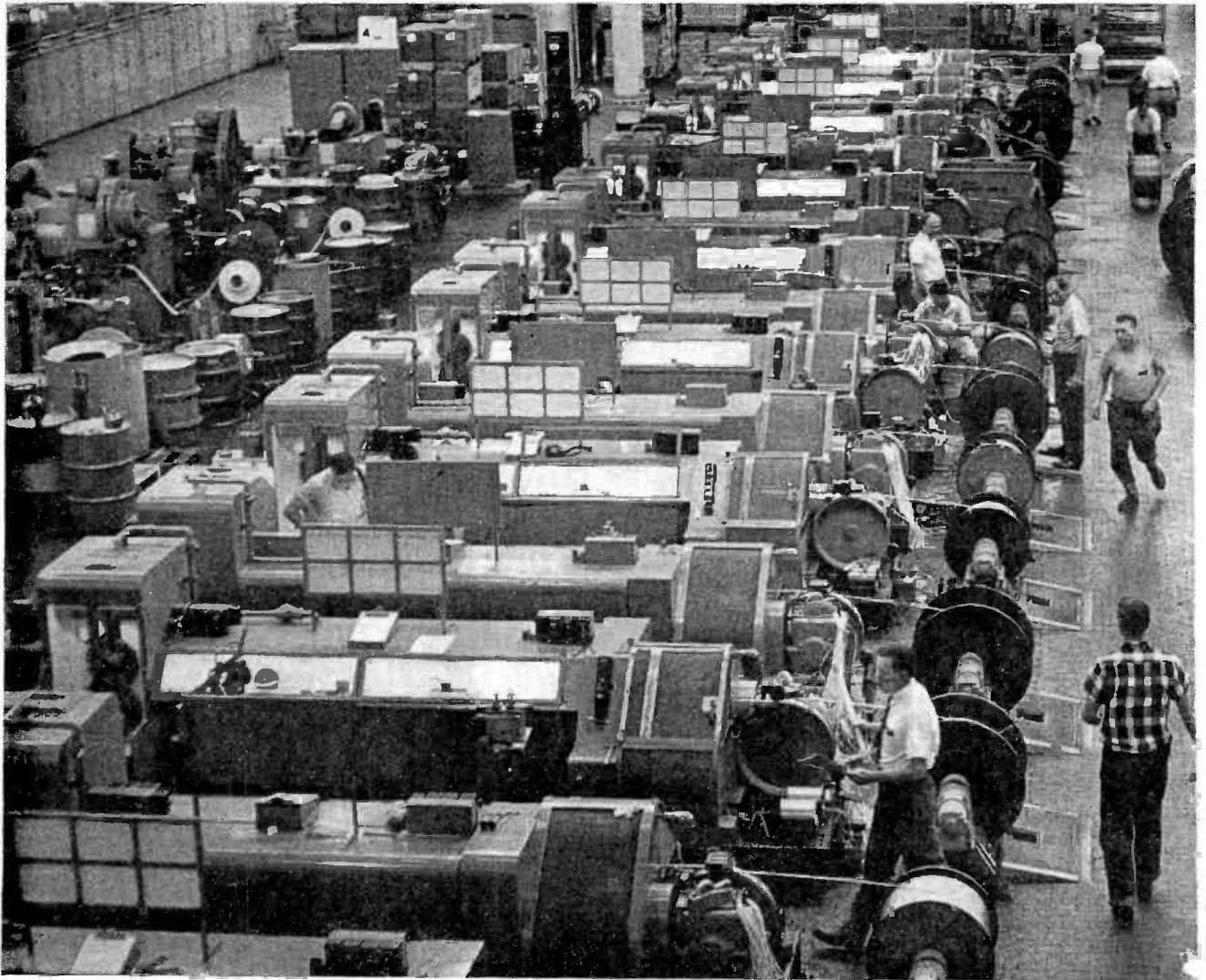
9,300 conversations can be transmitted simultaneously on a new 12-tube coaxial cable made at Western Electric's Baltimore Works. Laid underground, this cable will be an integral part of an almost indestructible communications network that is being installed across America. To make sure the cable meets the high quality standards of the Bell System, extensive quality charts like those on the cable machines above are kept for each cable production line.
