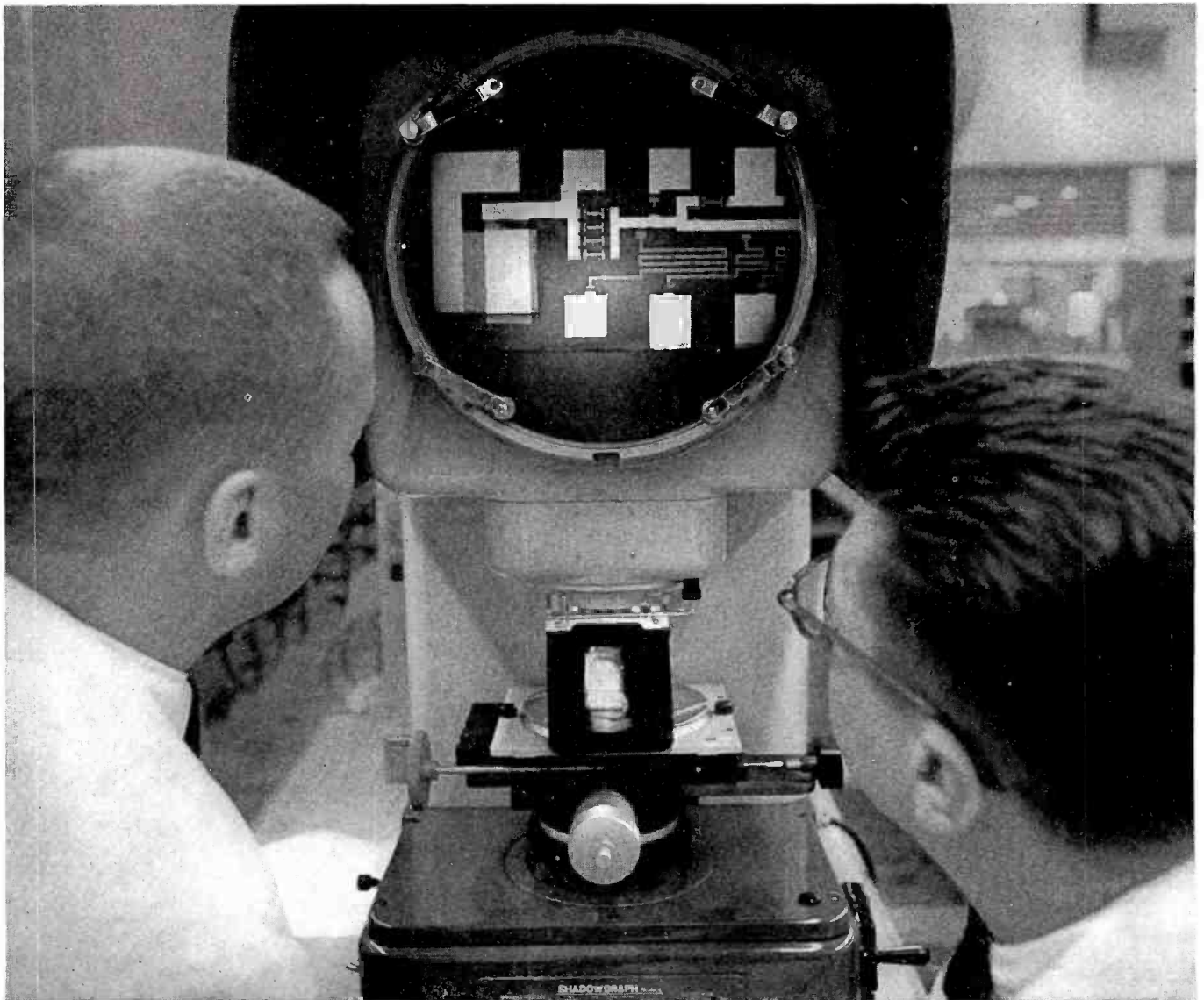
At Western Electric's Allentown Works, W.E. engineer Dave Ports (left) and William Moberg of Bell Laboratories examine a greatly magnified thin film circuit. This product is the result of Western Electric-Bell Laboratories teamwork... will help bring further miniaturization and more economical manufacture of telephone components.
