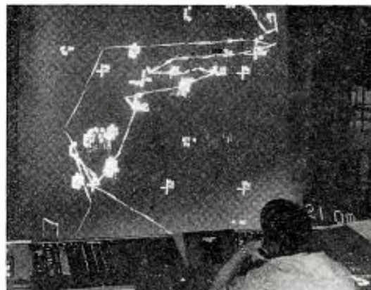
SAGE PROJECTION SCREEN presents situation display to Sector Commander at Semi-Automatic Ground Environment direction center—allowing a potential enemy air attack to be quickly detected and missiles and fighter aircraft directed to selected targets.
