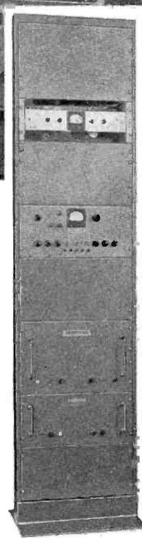
PHILCO TLR-6 TRANSMITTER Consists of transmitter chassis and associated power supplies. All operating controls and most frequently used maintenance controls are conveniently located on front panel.
