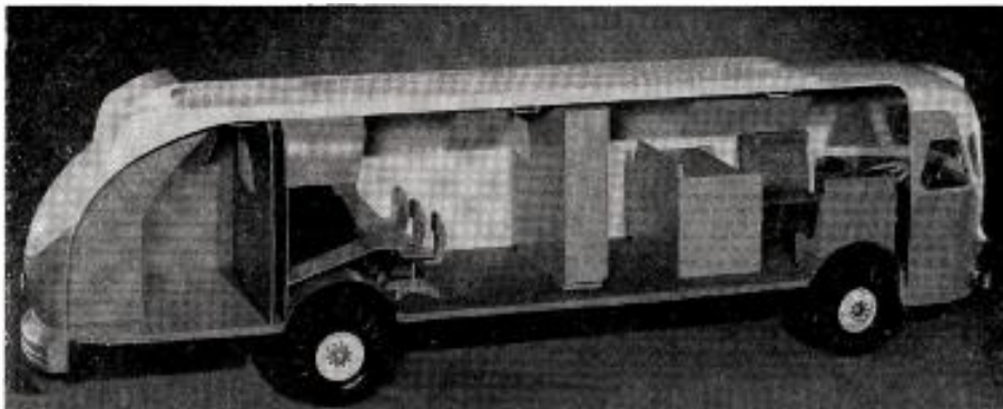
AMPEX CORP. of Redwood City, Calif., is developing a self-contained VR-1000 videotape recorder mobile unit. In the scale model above the recorder console faces seats behind the driver's position; behind it are equipment racks and, over rear wheels, control panels, monitors and other equipment. Generator, air conditioning and storage bins are carried in the rear compartment. Variations of the design also are being considered.
