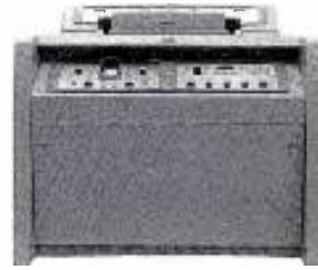
VR-1000 Videotape Recorder First commercially available Videotape Recorder. Magnetically records what the camera "sees", either black and white or color. Playbacks look "live".
