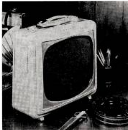
"BRIEF CASE" PORTABLE bears the name "Slender Seventeen" and has Scan-Tenna rotating handle antenna.
