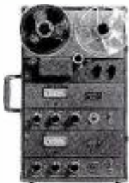
MODEL 601-2 Portable Magnetic Tape Recorder First professional quality portable. Lightweight and compact, it meets rigid standards of audio and mechanical performance.
