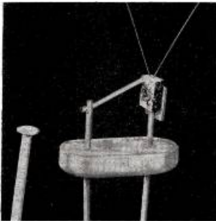
RAYTHEON'S mighty though minuscule "spacistor" here is attached to the boat-shaped mount of a transistor, a unit it may make obsolete. At left is a straight pin. The experimental spacistor, according to its developer, promises to combine many of the best properties of the vacuum tube and the transistor.
