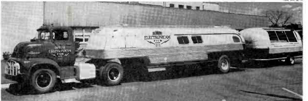
DUMONT'S new mobile Electronicam film system is contained in two functional trailers (bottom), readily moved from stage to stage and set to set. The smaller unit goes on stage as the control center while the larger one remains outside during film production. In the control-room trailer (top), the equipment is given a final check by Keeton Arnett (seated), vice president of Allen B. DuMont Labs, and John Auld, manager of operations, Electronicam Div., before unit leaves the Clifton, N. J., plant for use in Hollywood.
