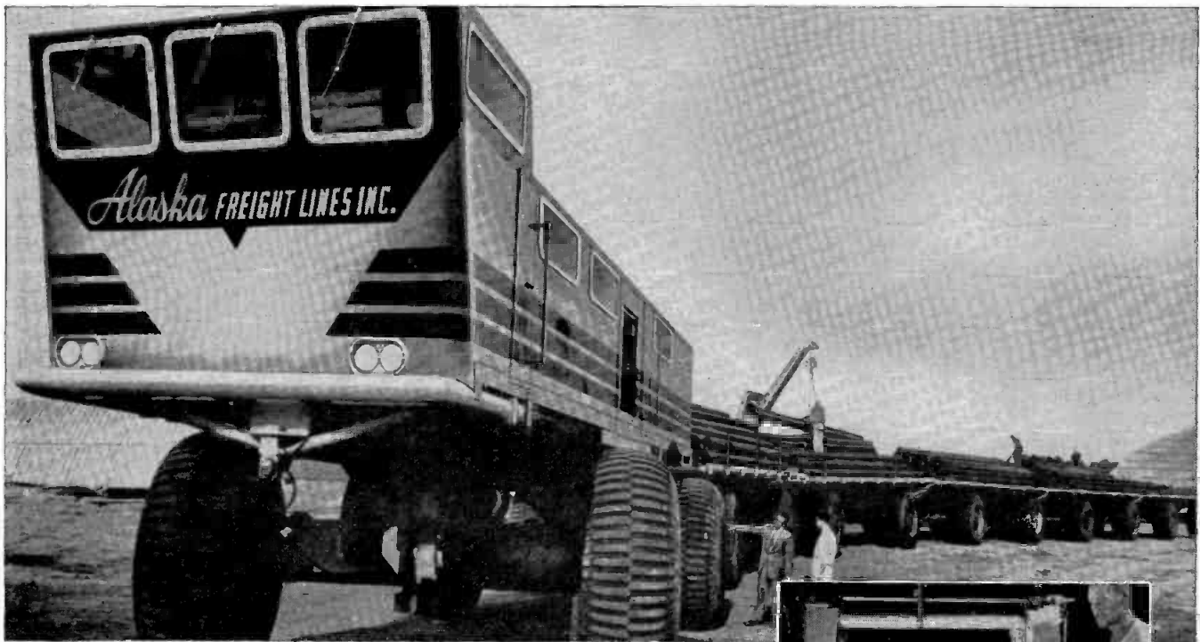
Let It Snow. This eye-popping "Sno-Freighter," built by one of our customers for Alaska Freight Lines, Inc., operates over snow, ice and bulldozed trails. Each wheel in the 6-unit train is driven with its own electric motor. The 7-foot-high tubeless tires are 38 inches wide at the base, and the Sno-Freighter can wade through 6-foot-deep water without damage. USS steels played an important part in this amazing machine, including USS Shelby Seamless Tubing for the vital car coupling system.
