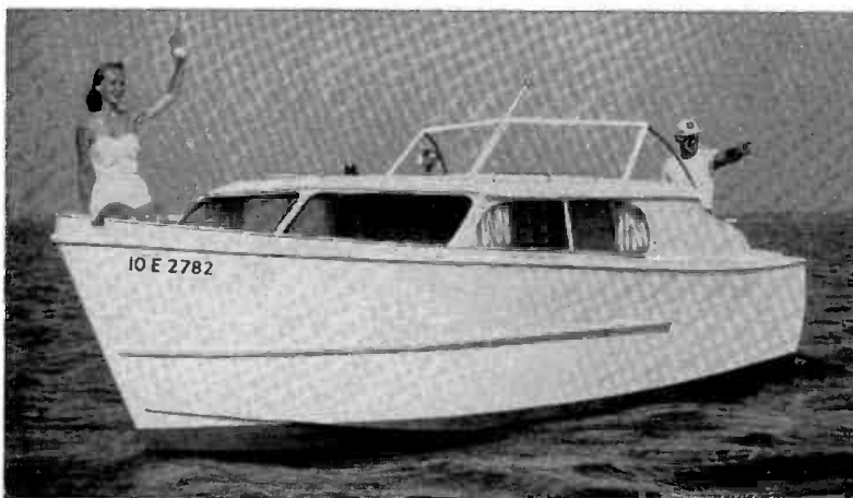
Beautiful—And Safe. This handsome boat is possibly the safest pleasure boat ever made. With welded construction, gasoline and bilge areas can be completely separated, eliminating the most common cause of boat disasters: fire. The boat is made from USS COR-TEN Steel, which is much stronger and more resistant to corrosion than carbon steel.
