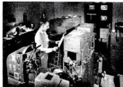
Projection room has three film projectors; two Teloprotectors with a capacity of 12 slides each; and Teloprotector which holds 10 telap cards.
