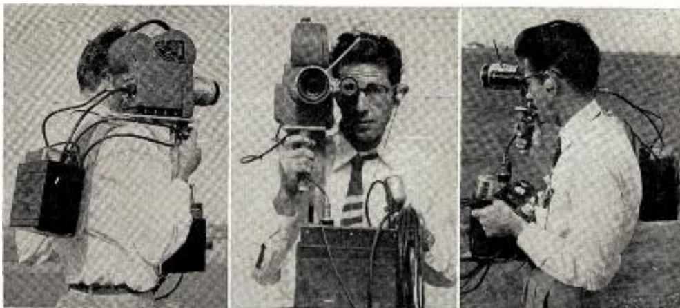
KWTV (TV) staff photographer Bill Horton demonstrates his one-man rig for sound-on-film news coverage which does away with necessity of tripod arrangement.
