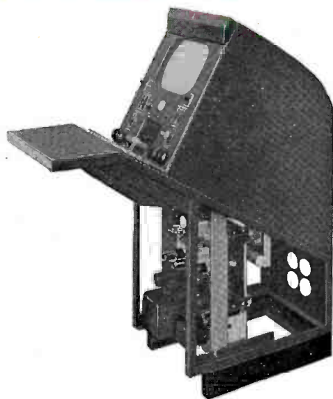
The TS-11A Switcher is supplied with an RCA console housing (MI-26266-B), a TM-68 master monitor and power supplies to form a complete versatile system.
