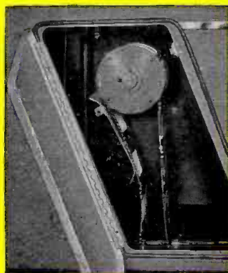
Telop III...interior view of automatic slide holder which accommodates 4" x 5" opaque slides...One lens...no registration problem...no keystoneing.
