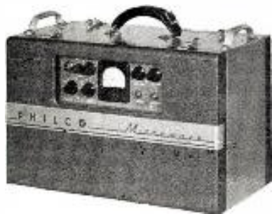
Transmitter Control and Power Supply
