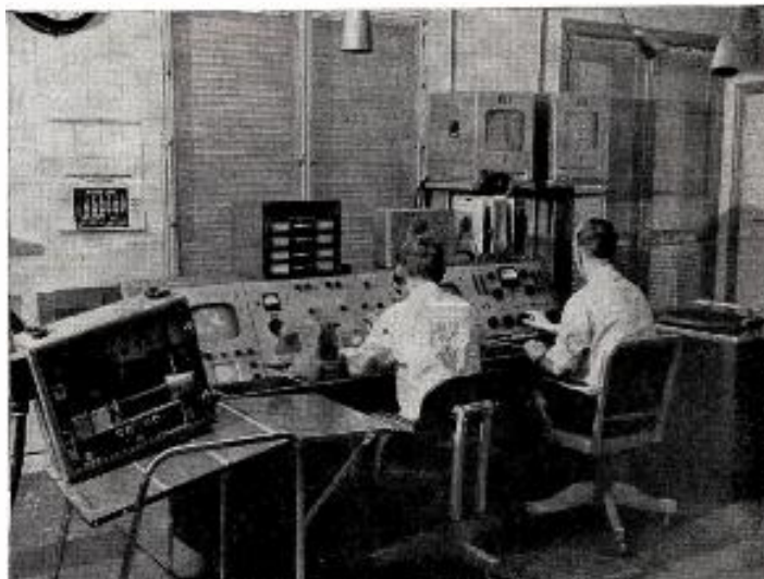
Two engineers control WNAO's entire program schedule—slides, film, studio and network—with Federal Transmitter Control Console and Poly-Efex Scanner providing complete transmitter supervisory control and audio/video switching. Scanner includes 2 slide sources, four-channel video switcher and "special effects" section.
