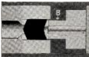
2) Outer ram "B" presses on the billet, holding it firmly in place.
