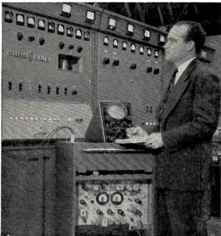
Jim Tillman measures envelope delay through a G-E 12 KW Klystron UHF transmitter.
