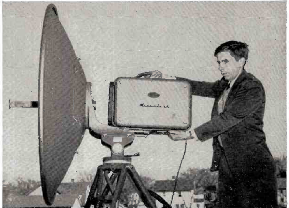
MICROLINK's ease of assembly is shown by a Raytheon engineer who fits the transmitting unit to its parabola. Machined guides assure
