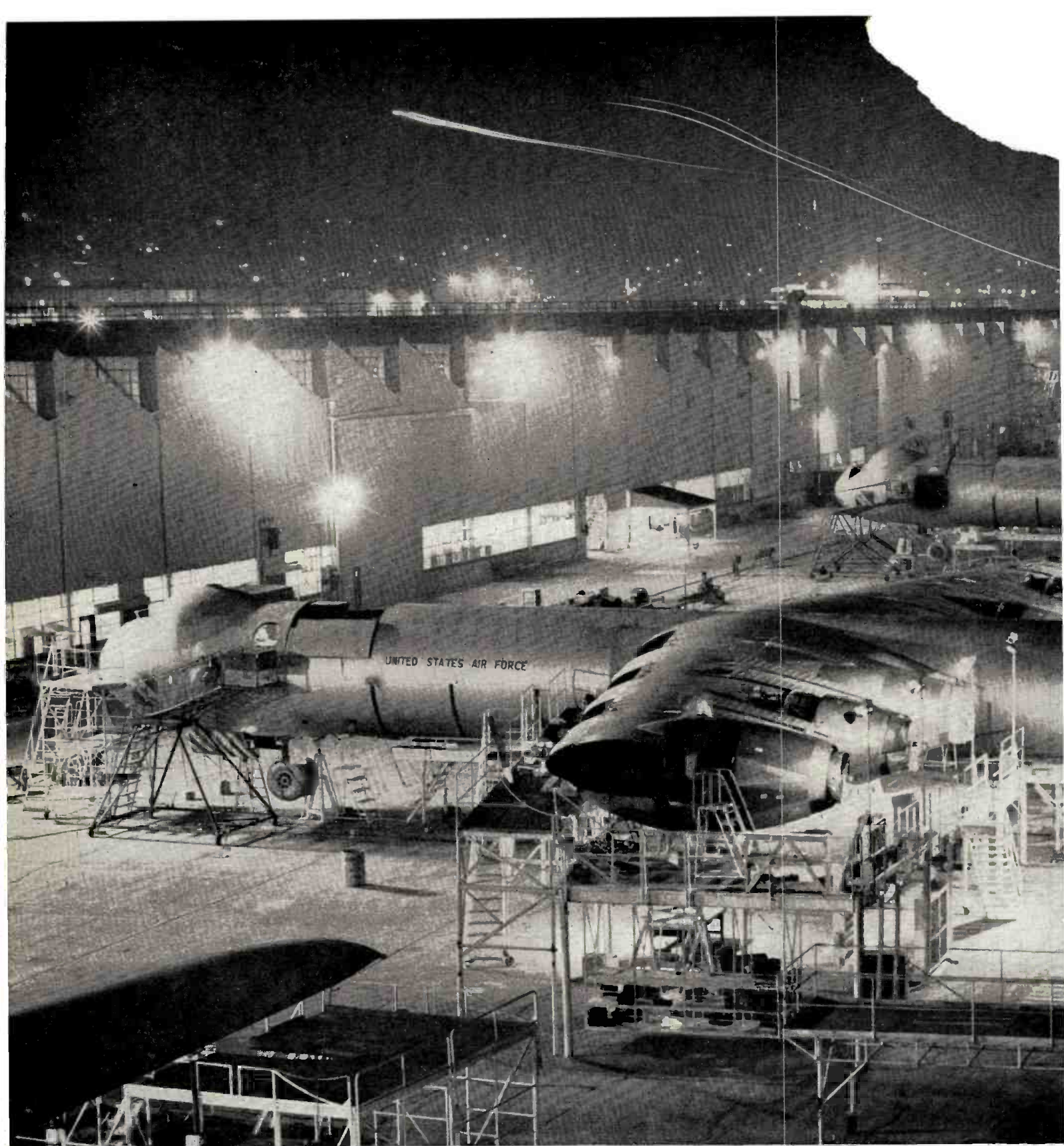
INSTALLING JET ENGINES IN B-36's, PICTURE TAKEN AT CONSOLIDATED VULTEE PLANT NO. 2 AT 1:30 A. M.
