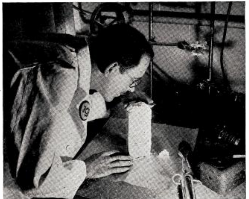
This block of luminescent material, energized by ultraviolet light, provided illumination for this photograph.
