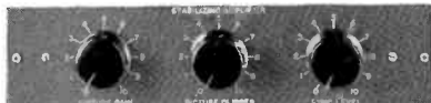
Stabilizing Amplifier Control, MI-26250. Includes three potentiometers. Controls: (1) picture gain; (2) picture clipper; (3) sync level in stabilizing amplifier.
