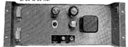
Current Regulator, MI-26090. Maintains constant current in focus coil of Studio Camera TK-10A. Current can be adjusted over a range of 65 to 85 ma.
