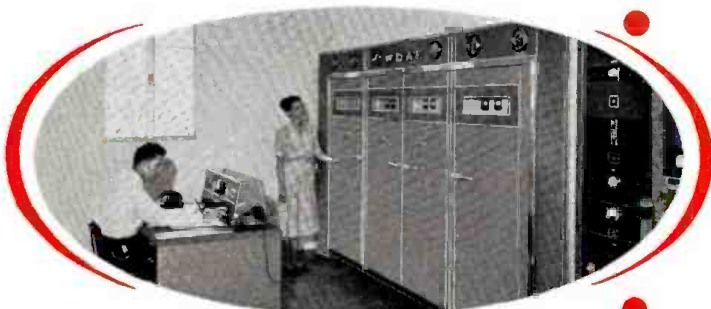
WDAE—TAMPA —Owned and operated by the Tampa Daily Times, the city's oldest station has been on the air since 1922. In recent complete modernization program, WDAE officials selected the General Electric 5 kw AM transmitter (above).
