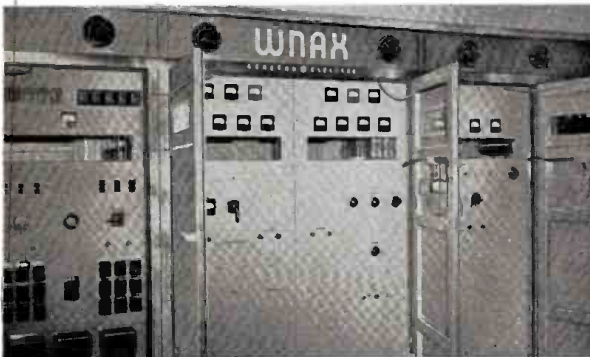
WYAX—YANKTON —On the air since 1926, this South Dakota station recently modernized its broadcast facilities, installing a General Electric 5 kw AM transmitter.
