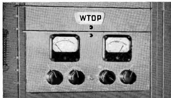
G-E Limiting Amplifier at the 50,000 watt transmitter of WTOP, Washington, D. C.
