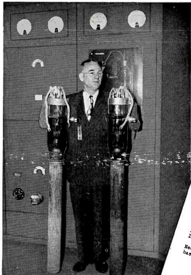
Chief Engineer M. J. Minor of WBT, Charlotte, N. C., retires two Federal 862-A tubes after more than 30,000 hours of service.
