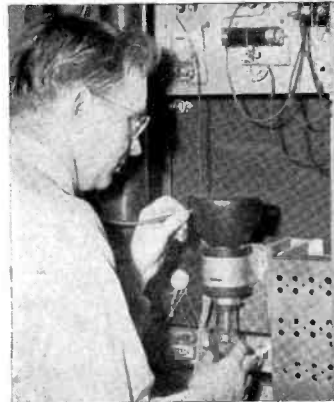
L. E. Swedlund, senior engineer in charge of projection tube development at RCA's Lancaster, Pa., plant, adjusts new "Flying Spot" tube in a video signal generator.
