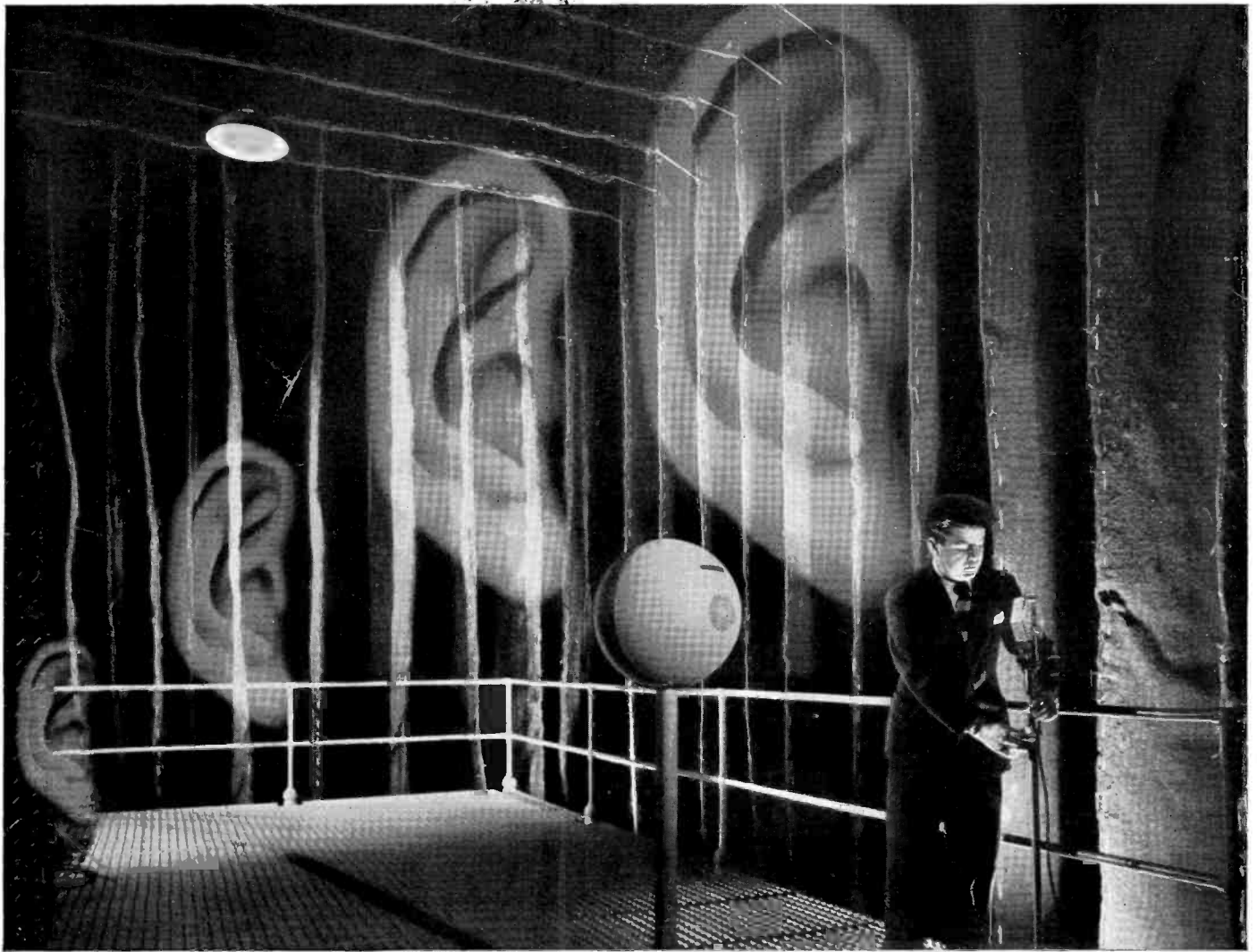
RCA Laboratories' "Chamber of Silence"—proving ground of tonal quality in radio and television instruments.
