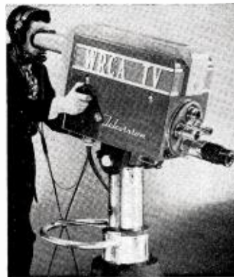
This new studio type Image Orthicon television camera requires only one-tenth the amount of light needed by iconoscope cameras, according to RCA-Engineering Products Dept. of RCA Victor, which developed it.
