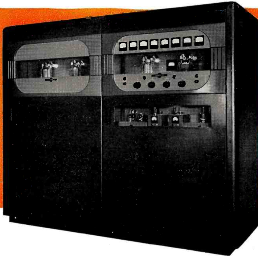
The 20T 1 kw AM Transmitter
