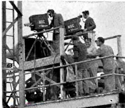
WNBT —Two RCA image-orthicon cameras, operated from a specially erected television platform, help bring the Navy-Duke football game to televiewers in the New York area.
