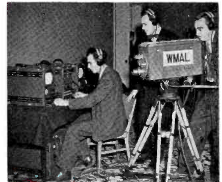
WMAL , Washington, D. C., picks up an indoor event with its new image-orthicon camera. Monitoring is done at the easy-to-carry, suitcase-type control units.
