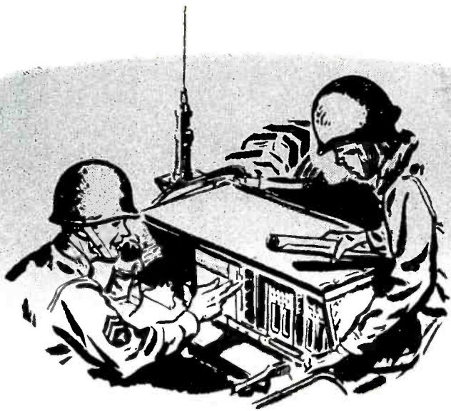
Bell Laboratories designed and Western Electric furnished more than 139,000 multi-channel FM receivers and 74,000 multi-channel FM transmitters for use by the Armored Forces and Artillery.
