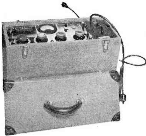
↑ THE GATES 3 CHANNEL PORTABLE REMOTE AMPLIFIER FOR ALTERNATING CURRENT OR BATTERIES.
