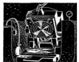
FINALLY , each disc is molded in finegrained, flexible, moisture proof Vinylite, resulting in high fidelity, elimination of background noise, and long wear.
