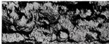
Surface of etched nickel, as seen by the new RCA Electron Scanning Microscope.
