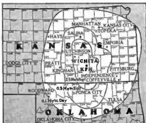
Clara D. Gillet Computer Field Strength Distribution Based on Performance and Previous Survey Measurements—5000 Watts Day and Night—October 1941
