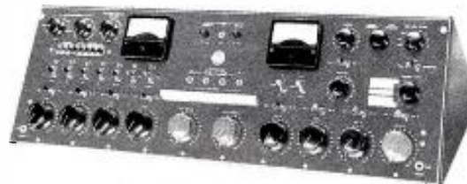
THE "DUAL-CHANNEL" AUDIO CONSOLE, BC-6A. Twenty-Two Inputs—10 microphones, 2 turntables, 2 tape, 2 film, 5 remote lines, 1 network. Dual or single channel operation with "split-mixer" faders. Master fader controls both channels simultaneously. Ideal for binaural broadcasting. Nine mixer positions. Two built-in power supplies (one for each channel) for greater reliability. Two monitoring channels, one for program monitoring and talkback, one for cueing and feeding background to studios. Convenient script rack.
