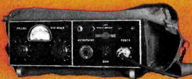
212U 2-channel remote amplifier (212Y remote amplifier combined with 60H mixer)
