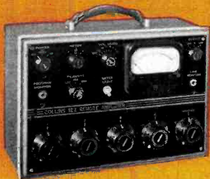
12Z-2 remote amplifier (input impedance 30/50 ohms) and 12Z-3 (input impedance 200/250 ohms)
