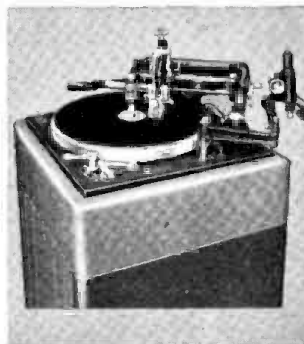
4. Presto 8-N recorder, the finest recording turntable made by Presto. Used by the larger stations in U. S. and Canada. Records made on the 8-N reproduce uniformly range 50-9000 C. P. S. Noise level -50 db.
