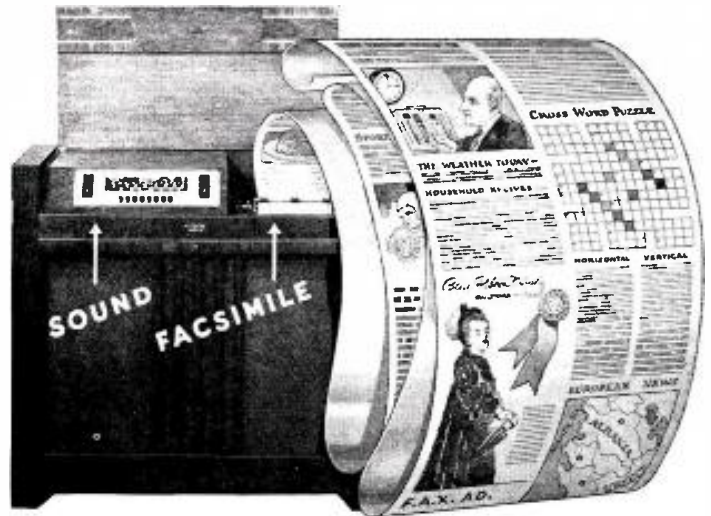
One of several types of instruments for receiving both sound and facsimile programs separately or together over one wave band. Drawing is from typical program of news and features.
