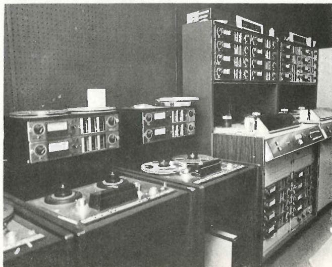
Part of the stereo, 4, 8 and 16 track recording equipment at Toronto Sound Studios.
