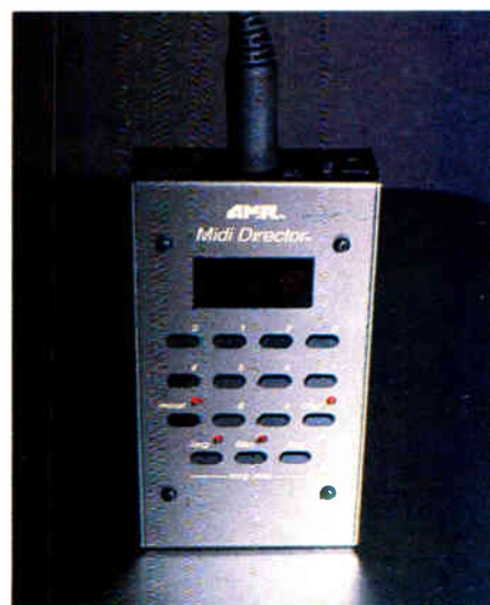
The AMR MIDI Manager offers inexpensive remote control for MIDI synths, sequencers and drum machines.
