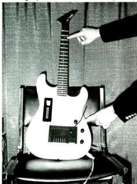
Beetle's Quantar MIDI guitar controller system is now fully self-contained.
