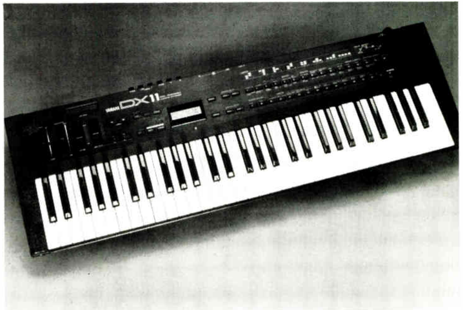
Yamaha's new DXII is basically a TX8IZ with a keyboard and a few additional editing features.
