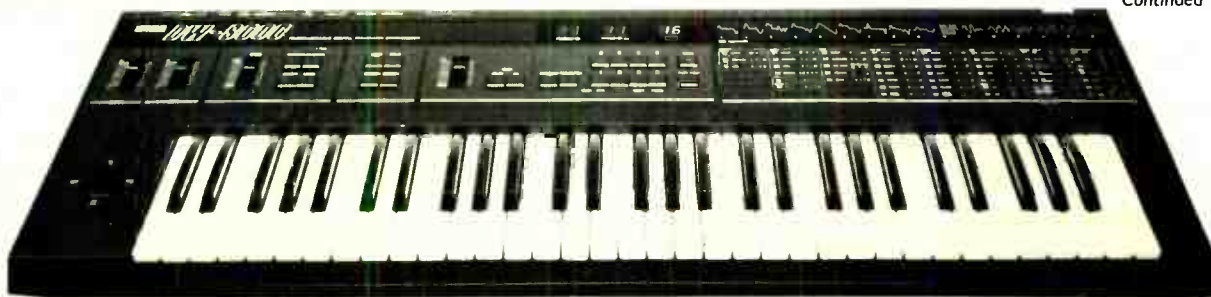
Korg's DW6000 and DW8000 synths utilize DWGS (digital waveform generator system), a new digital method of sound generation.
