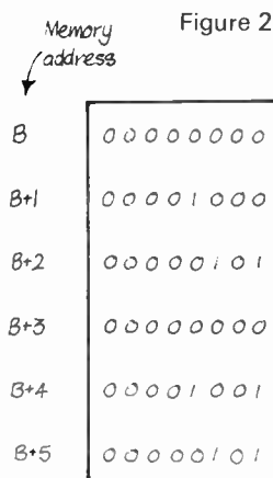
A "lock-up table" (above) which allows the root of major and minor triads to be identified from the lowest note and the entry number derived from the table in Figure 1. On the right are the equivalent binary numbers, showing how the table may be stored in consecutive memory locations, starting at any convenient address (denoted by B). B is known as the "base address" of the lock-up table, and the entry number is equal to B + 1.
