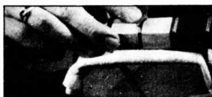
Filing fret ends with three-cornered file
