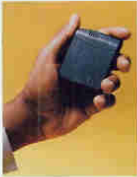
The PPM is a pager-sized device that will be carried by consumers in order to detect inaudible station identification codes that broadcasters embed in the audio portion of their programs.
