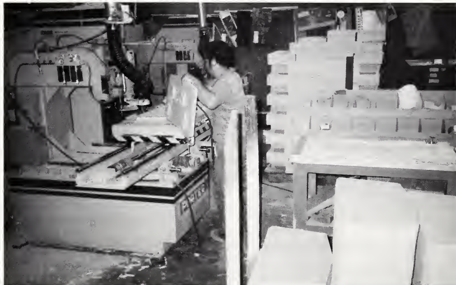
Then the holes for the joysticks and buttons are cut, as you see here, as the control panel prepared.
