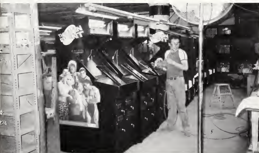
The Main Event's side decals must be applied and the marquees must be put in place, and that's what is happening in this photo.
