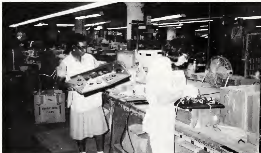
Wiring the power supply assemblies comes next; and then, as you see here, the control panel must be assembled. Buttons and joysticks are carefully wired after the control panel overlay applied.
