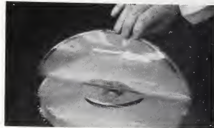
Technician removes a videodisk replica from replicating machine.
