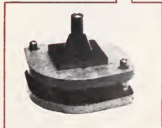
Fabelou ● Tool for precise cutting of center & edge for 7" records, in one operation
