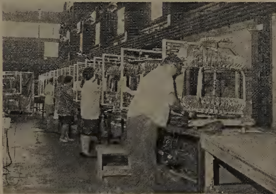
The revolving film magazines for the forty-selection audio visual machines are assembled on this line at the factory.
