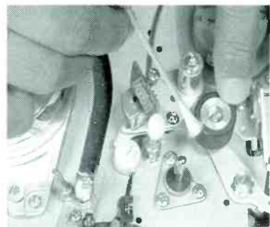
In a still from the Alesis/EMTEC Pro Media instructional video "Care And Feeding Of Your Adat," a technician demonstrates the proper way to clean the machine's tape path.
