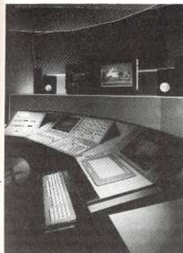
Digital Scenaria. Solid State Logic's Scenaria is a digital postproduction system complete with 38-channel audio mixer, 24-track random access audio recorder, multitrack audio editor, multiple machine controller, automated routing system, and random-access video. Since its debut in April SSL has sold more than 15 of the systems to major facilities in the U.S. market. A complete Scenaria setup lists for about $250,000.
