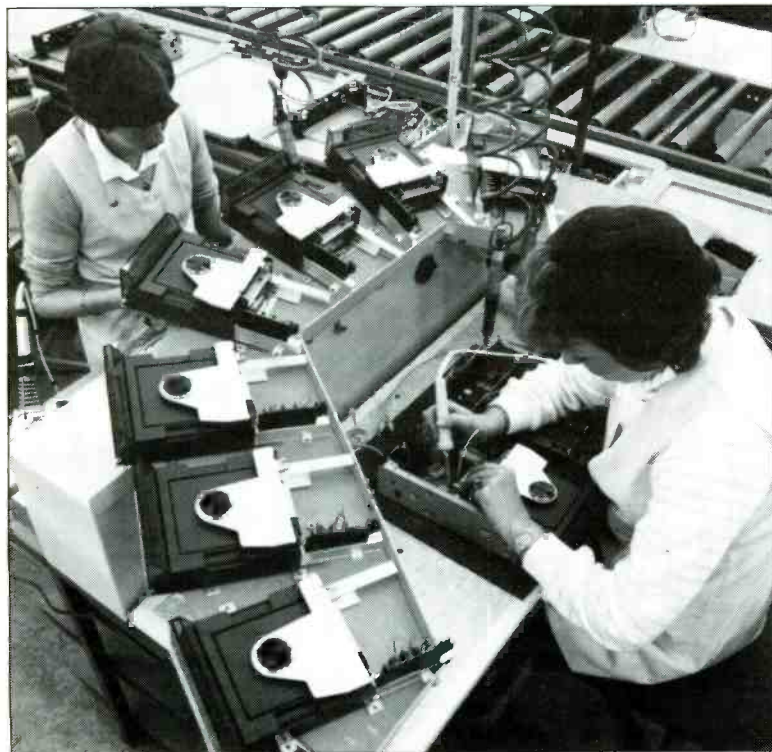
Factory workers assemble Philips CD 300 players on a production line
