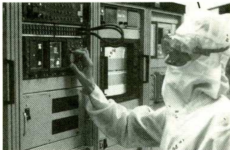
In the clean room during the transfer process, an operator creates using the cutting machine to transfer audio and video signals from D-2 tape to a glass master.
