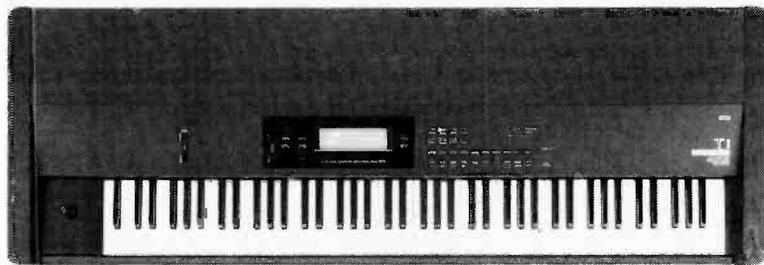
**Korg Workstation Expansion.** Korg introduced the T1 (above), part of its T Series of 8 megabyte ROM keyboards offering 16 bit sounds, a PCM card slot and program card slot, and 1 megabyte RAM. Based on the M1, the series also boasts a 50,000-note internal sequencer as well as a feature that allows programs to be saved and loaded to the internal disk drive, which uses 3 1/2-inch disks. Contact Korg at 516-333-9100.
